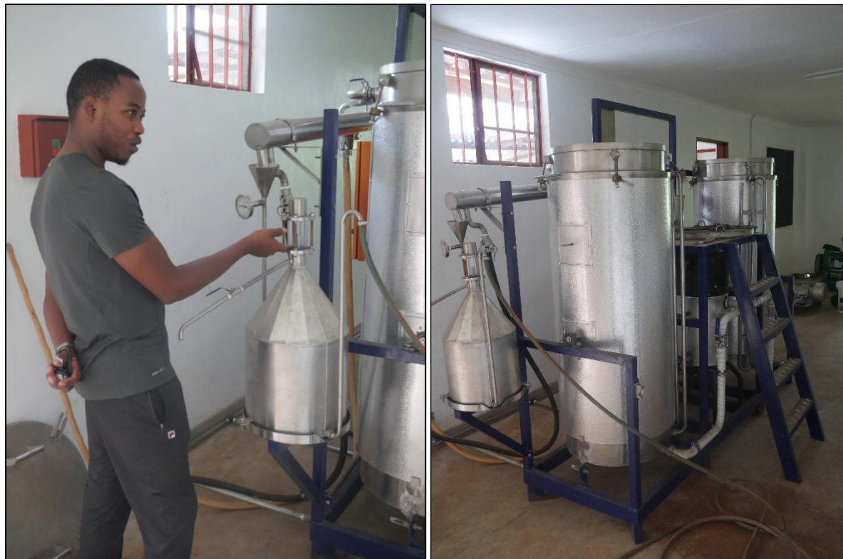
Figure 2: The larger distillation equipment (100kg - right) with project manager, Ibrahim Mitole, explaining how the oils are produced (left)
