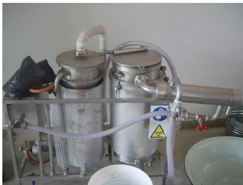
Figure 3: The smaller distillation equipment (10kg) for tester production of oils from plant materials
